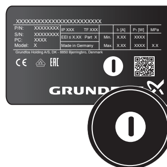
Identifying the master pump head on the nameplate
