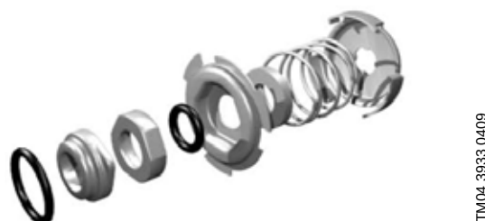
Fig. 14 Exploded view of shaft seal
