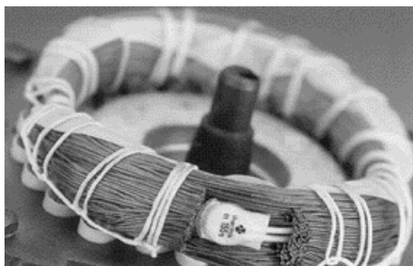
Thermal switch incorporated in windings
