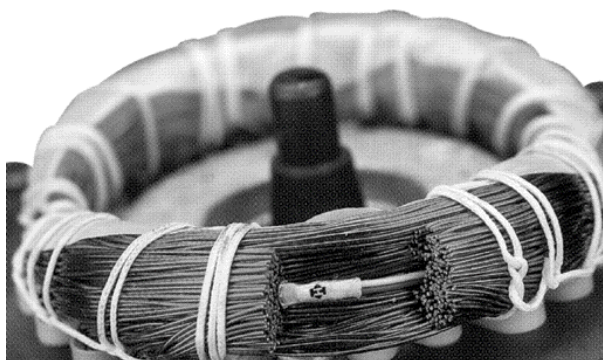
PTC sensor incorporated in windings
